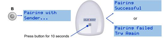
**IMPORTANT!** Do not press the sender button except when performing the pairing process. If it is pressed for more than one second the pairing may be lost and the display shows a 'Lost Signal' message (see Trouble Shooting). To correct, either reset the sender by removing and refitting the batteries or use the above procedure to reset the pairing.
