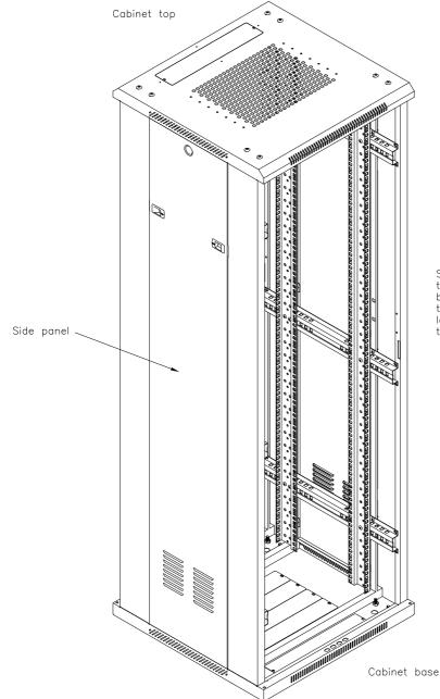
Stage 6. Locate the side panel by fitting the locating pins into the 2 slots in the base unit, then lean the side panel into the cabinet making sure that the plastic latches engage securely into the slots in the side frames.
