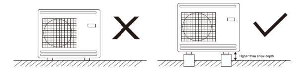
The heat pump should not be positioned next to sensitive walls, for example, next to a bedroom. Also ensure that the placement does not inconvenience the neighbours. The heat pumps must not be placed so that recirculation of the outdoor air can occur; this causes lower output and impaired efficiency.
