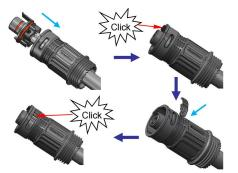
Insert Seal and Clamp Finger into socket ,then tighten the nut , torque 8+/-2N·m.
