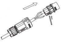
Push the threaded sleeve into the socket, tighten up the cap on the terminal.
