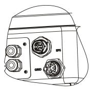
Remove the ON-GRID connector: Press the bayonet out of the slot with a small screwdriver or the unlock tool and pull it out, or unscrew the threaded sleeve, then pull it out.
