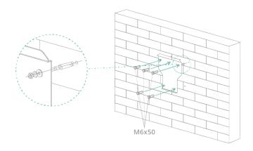
5. Mount the inverter onto the mounting bracket.
