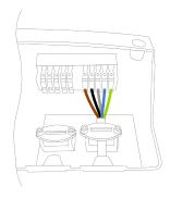
8. You must install a separate AC circuit-breaker per inverter in order to ensure that it is adequately protected and can be safely disconnected under load. Please follow local legislation.
