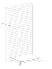
2. Stack the battery modules on the base making sure they are flush to the wall. Adjust the feet to make sure they are flush to the wall and level left and right. Once all of the battery packs are in place use the template to determine the location of the wall bolts. Ensure the template is level and completely flush to the wall.
