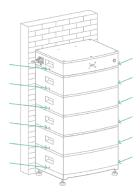
1. Connect the cable to the battery and the other end to the inverter. Ensure that the grommeted end of the cable is the inverter end. Push the plug until there is a click, lock in place using the red tab.
