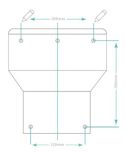
**4.** Drill 5 holes at the marked positions, at least 75mm deep. Fix the mounting bracket to the wall using 5 x M6x50 expansion bolts.
