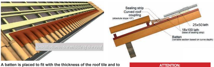
A batten is placed to fit with the thickness of the roof tile and to provide a flat base for the sealing strip.
