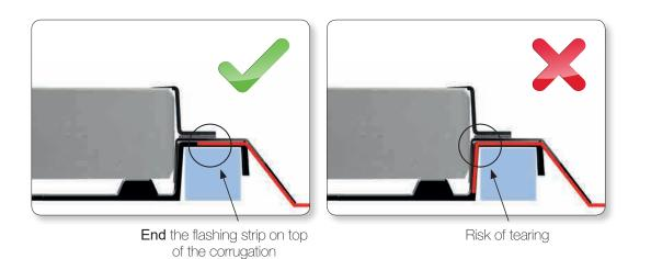
ATTENTION: IN BOTH CASES, THE FLEXIBLE STRIP CAUGHT BETWEEN THE FLASHING AND THE CORRUGATION OF THE GSE PANEL MUST BE POSITIONED ON TOP OF THE CORRUGATION TO PREVENT THE RISK OF TEARING.
