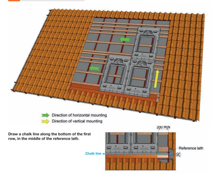
Interlock the plastic frames from the right to the left side (left to right is also possible - check that the interlocking is well done)
