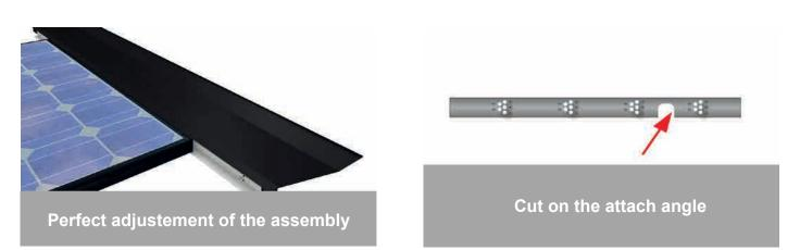
Place the top junction flashing, having applied beforehand two PU glue joints on the covered top flashing area. The connecting piece must overlap with the top flashing with at least 100 mm. The gap between the top flashings should not exceed 160 mm.
