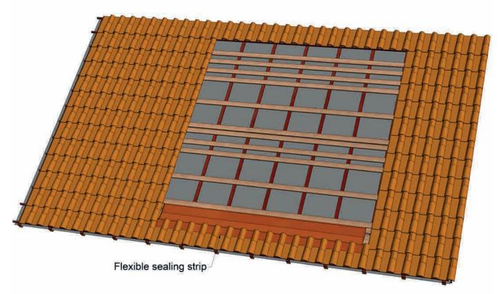
The sealing strip is laid out to link up with the bottom part of the roofing (PV array in the middle of the roofing).
