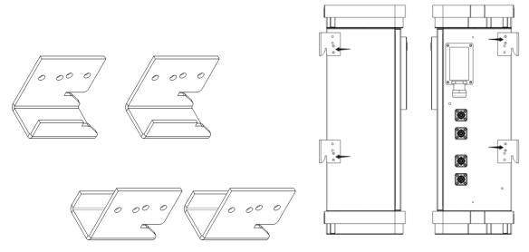
1. Install the wall brackets to the main body and slot the battery on the support frame
