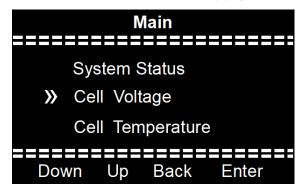
Use UP and DOWN key to navigate. Press ENTER to select Cell Voltage to enter the Cell Voltage page.
