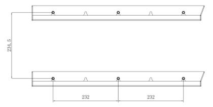
5. Take the four wall holders. The left and right holders are different and the side with a crevice is always facing down.
