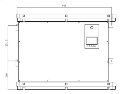
5. Align the four stand holders with the expansion screws, tighten the expansion screws until the battery module is secure.
