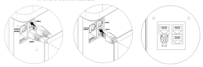
3. If you have more modules, repeat the second step and make sure the DIP switch address increases in sequence.
