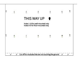
3. Mark the number 1 - 10 holes on the wall according to the drill template. Drill those holes to at least 65mm deep with a drilling machine and install the expansion screws. Minimum of 6 holes are required as shown on the photo below. If it is not secure enough, you can drill all 10 holes as marked.
