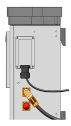
Insert the black end of the quick plug power cable connector into the upper black socket, connect the other end to the hybrid inverter negative pole, and cover the remaining sockets with plastic sleeves.
