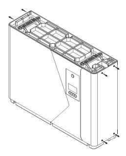
Placing both hands firmly on both sides of the outer cover, slowly pull towards you to separatee the top half of the cover from the battery.
