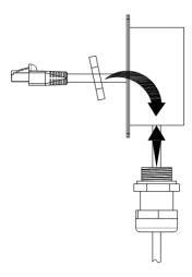
3. Plug the network cable into the CAN&RS485 port.
