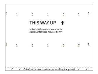
3. Mark holes on the wall at positions A, B, C, D as shown on the drill template. Remove the drill template and drill holes of at least 65mm deep and install the expansion screws.
