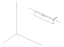
2. Align the drill template to the horizontal line and make sure that it does not move.
