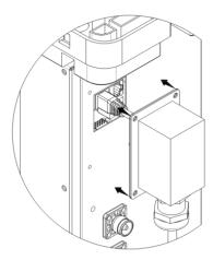
5. Connect the other end of the communication cable to the hybrid inverter.
