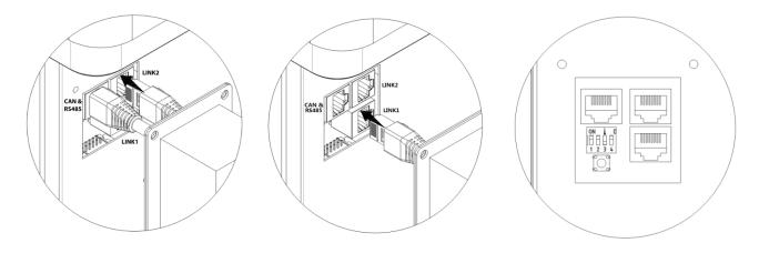
2. If there is a third module, plug one end of the network cable into the LINK2 socket of the secondary module and the other end into port LINK1 of the third module and turn the DIP switch of the third module to 3.
