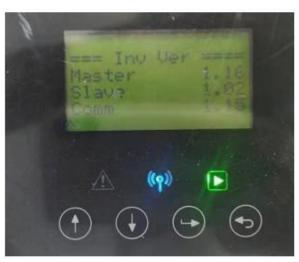
7. Turn on AC &DC breaker. If you updated the HMI, long press the "enter" and click "set" to turn on the inverter. Make sure the inverter can enter **Normal State**.
