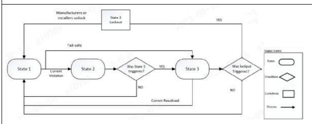
Ginlong G100 CLS was designed with a fail safe mechanism according to G100 Issue 2 2023, ensuring that in the event of communication failure or loss of source in any component, reducing the component generation to zero.
