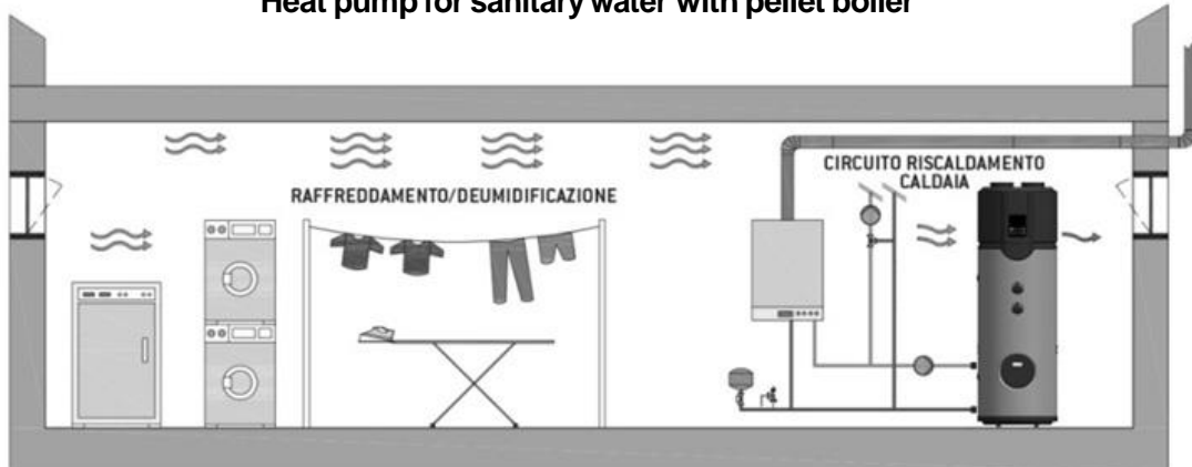
Heat pump for sanitary water with wall-mounted gas boiler
