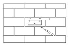
• Drill holes with electric drill, make sure the holes are at least 50mm deep, and then tighten the expansion tubes.
