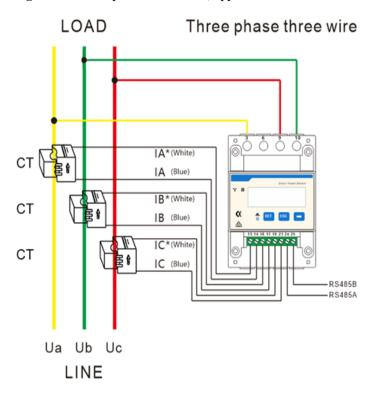
Figure 4-2 Three-phase three-wire (supported model: DTSU666-H 250 A/50 mA)
