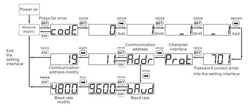
When modify digits," (ET)" can be used as cursor shift button; "(ET)" is "add"button; "(ESC)" represents exiting the setting interface or switch to the character interface from digit modification interface, restarting adding from zero after setting the digits to be the maximum value.
