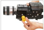
Slide the camera onto the quick release camera platform and press the red lever to lock it.
