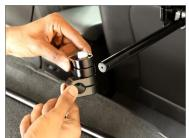
After inserting the 360° Houdini Rod Clamp, insert black anodized speed rail (3ft length) and secure it properly with the help of the Allen key.
