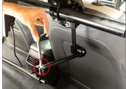
Black anodized speed rail (3ft length) with 360° houdini rod clamp are properly secured, as shown in the image.
