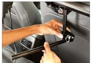
After inserting the rigging rod (250mm), tighten it with the help of Allen Key. Then insert the 360° Houdini rod clamp into it, as shown in the image.
