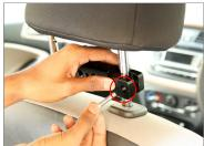
After inserting the bolt, properly secure the headrest on the backseat with the help of the Allen key, and same step is to be followed on the other side as well, as shown in the image.
