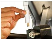
After inserting the baby pin, secure it properly with the help of the Allen key, as shown in the image.
