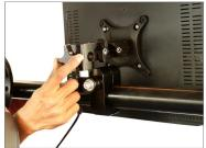
Attach the rigging road clamp to the round cheese plate by matching it with the threads, then secure it properly with the help of Allen Key.
