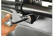
To secure the rigging road clamp, insert the rigging road 180mm in it and secure it with the help of Allen key.
