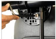
Then insert 360° Houdini Rod Clamp into the Rigging Rod (180mm) and secure it properly with the help of the Allen key, and then insert rigging rod (250mm) into it.
