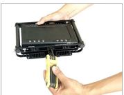
Mount the monitor cage into the stand and tighten the provided knob to secure it properly.
