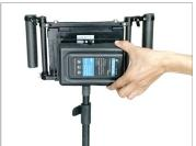
• Push the button of the top battery plate and remove the v-mount Battery.
