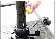
• Insert seat support side arm into the holder, then insert seat rod and tighten knob as shown in the image.
