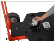
Place the Euro Adapter by carefully aligning the holes on dolly. Then tighten the allen bolts back to secure it properly on the base.
