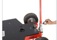
Position dual Steering Push/Pull Bar on the steering rod mount located on rear axle of dolly. Connect them properly by locking with provided knob.
