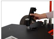
Insert Seat Rod into Z-Bracket and lock it securely with locking knob.
