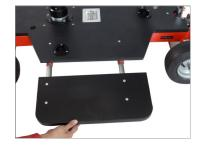
**NOTE:** Mounting of Euro Adapter enables fitting of various camera mounting accessories such as Bazooka, Risers, and other Adapters etc.
