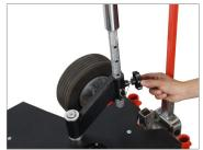
• Now attach the Chair with Z-Bracket and tighten the provided knob to fix it accurately.
