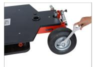
**NOTE:** By correctly using Steering Push/Pull Bars, it is possible to maneuver Quad Dolly with extreme precision.
