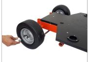
• Detach the wheel from the quad dolly and insert the provided bush.
