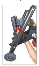
• Then, attach the other end of battery (marked with arrow) wire to the LCD Monitor.
