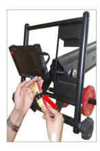
Finally, insert the other end of long RCA male jack in to camera port.
