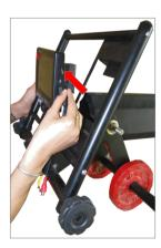
• Now, connect the Female RCA Jacks of short cable with male RCA jack of long cable as shown in the picture.
