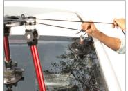
• Adjust the rope with the help of the push-pin button of the hook, as shown in the image.
