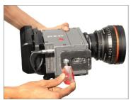
Pull the knob of the fluid head (Not Included), then slide and mount the camera (Not Included), as shown in the image.
