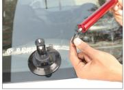
Screw the other end of the aluminum rod (30cm) onto the Ball Tilt head, and then tighten it.
