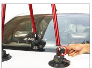
Screw the rods into the camera mounting platform and tighten them.
