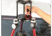
• Secure all the bolts using the Allen key.
