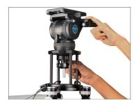
• Loosen the fluid head (Not Included) knob and then remove the plate.
