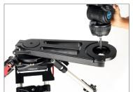
Insert the locking knob to the Fluid Head from the bottom and properly tighten it, as shown in the image.
