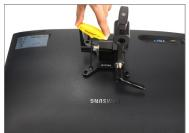
• The Monitor mount is completely attached to the monitor, as shown in the image.
