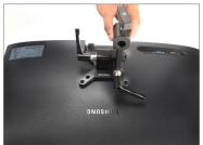
After inserting all screws, secure them using the Allen key.
