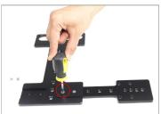
Similarly, attach the second side bracket to the base platform and tighten it with a screwdriver.
