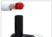
Lock the tube connector using the provided pins for better safety and security. Then connect another aluminum tube with the previous tube via tube connector.
