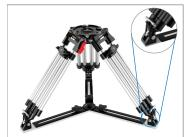
Now loosen the knobs of the foot spreader and extend its legs to full length to establish the lowest profile of the tripod, and then secure it by again tightening the knobs.
