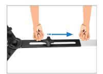
• Once extended, tighten the knobs properly.
