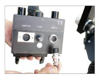
CAUTION: The power specification we have provided is as per 12volt. For this, we provide a 12volt/3A regulated power adapter. In case you use a voltage higher than 12V, it will affect the performance and life of the motor, and there is a high risk of the motor getting damaged.
