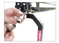
Attach the head cable to the cable connected to the gold pan tilt head for panning & tilting.
