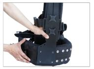
• Shift the bottom plate of the jacket from one side to the other and tighten all the bolts using an Allen key, as shown in the image.
