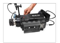
Slide the Camera onto the Fluid Head and properly lock with the help of the locking pin.
