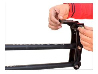
• Now attach the camera on quick release plate and secure it with provided screw.
