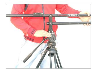
• Press the Pin on both jib arms to extend the length of jib. Tighten both the knobs to secure.
