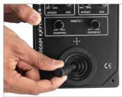
**Damping Control:** The damping control knob prevents the Head from stopping abruptly with a jerk, giving you smooth endings. The amount of damping is increased by rotating the damping knob clockwise.
