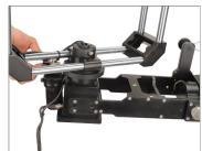
Set the direction of the Pan Tilt (Upward/ Downward) according to your requirement.
