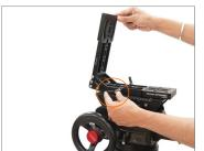
• To mount the camera on the wedge plate, screw the bolt onto the wedge plate.
