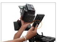
Align together the wedge plate screw and the camera thread. Then, tighten it with the help of an Allen key.
