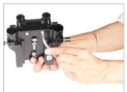
• Mount your Camera on the Base plate and secure the bolt using an Allen key.
