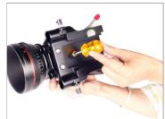
• Slide the base plate with the Camera mounted on it on the dovetail plate and press the Locking lever to secure it.
