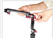
• Slide the Dovetail Quick Release plate on the threaded crossbar.
