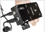
• Connect the electric plug of the 12v adapter wire to the universal adapter for generating the power-supply.
