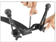
Place the middle feet at the center of the slider and then insert bolts, by matching the threads of the slider and the middle feet. Then tighten with an Allen key to secure.
