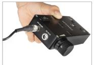
• Attach one end of the 12v adapter cable to the adapter.
