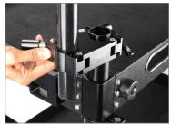
• The rods are properly secured to the Lateral clamp, as shown in the image.
