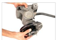
• After removing the Castle ring, mount the fluid head on the Mitchell plate.
