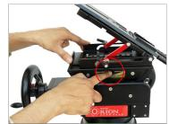
Mount the camera on the dovetail plate (Not included).
