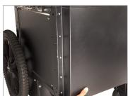
• Then insert the Allen bolt matching the holes, then tighten with the help of Allen key.
