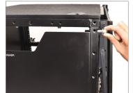
• Then, tighten the bolt with the help of an Allen Key, as shown in the image.
