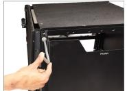
**NOTE**: Properly align the Back Panel and the Soundchief Cart together. Then insert the bolts and equally tighten them all. If the bolts are not all equally tightened, the threads can't be properly matched to that of the plate.
