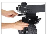
The brake wheel is properly attached to the Cart. Repeat the same process to attach the second wheel.
