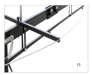
• Now attach one end of 14.3ft red cable to red hook on back side of jib (section 3) and align the red cable to the cable guide from top.
