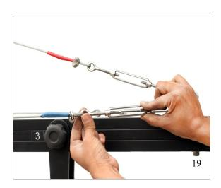
The jib arm can be locked (tilting) with the help of this knob.
