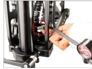
After attaching the washer of the air shocker to the air filling pump, pump the air using the latter.
