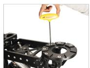
Also, align and match the side thread hole of the Mitchell platform and the Airwave V1060, and then insert and properly tighten the bolt using the Allen key.
