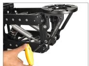
Now, the Mitchell platform has been properly attached to the Airwave V1060 in an over-slung manner.
