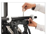
• Tighten both the bolts using an Allen key, as shown in the image.
