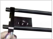
Insert the 300mm long rods into the front and back 15mm slots on the Cage bracket. Then insert the set of 200mm rods into the top rod holder of cage.
