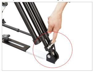
• In case of Dolly, Take out the bolt from the center of the dolly and spread it on floor. Then put the bolt back through the center of dolly again.
