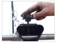
• Attach weights (Not supplied) to both ends of weight bar, secure with the help of closers.
