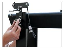
• Slide in 6th section to the rear to join the 5th section. Install the Allen screws to the joining holes of both the sections and tighten.
