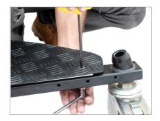
• Attach the legs of tripod stand with D-37 dolly as shown in the image.
