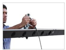
• Attach 14.5ft cable with Red Sleeves to hook attached on 1st section of jib and another end with 2nd hook attached to cable guide as shown below.
