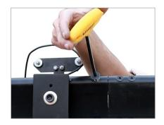
• Using the same approach insert 4th, 3rd and remaining sections to the joints and secure via bolts as shown below.
