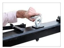
• Then attach 3 hooks to the hook that you attached (as per above image) with 1st section & 1 hook to 3rd section.
