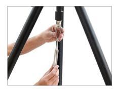
• Wire tensioner and safety chain setup should be properly aligned to ensure stability.
