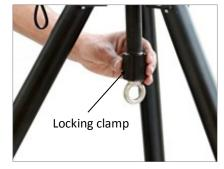
• To add stability to your Jib, attach wire tensioner with hook on Locking clamp, then attach one end of safety chain with hook on D-37 dolly and attach other end with wire tensioner as shown below.
