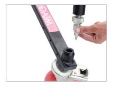
• Detach Locking clamp from central fork, mount central fork to tripod bowl, again attach Locking clamp for secure connection.
