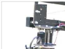
Removing Locking Pin from Central Post allows you to frame multi-dimensional tilting shots by using Control Handle.
