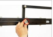
• Then tighten the bolt properly with the help of a wrench, and to attach section 5 to 4, loosen the bolt from section 4.
