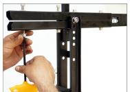
Section-5 has connecting bars attached with section-4 on both ends and then tighten them together using provided Allen key.
