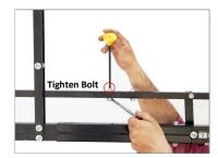
Continue the Arm build by sliding in section 2 onto section 3, and finally section 1 onto section 2.
