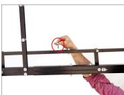
• Then tighten them together using provided Allen key and wrench as shown in the image.
