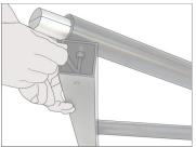
Now attach it with the Jointer of end foot and tighten the set screw properly with allen key. So that there is a minimum gap at the Jointer.
