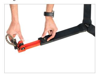
• Open the legs of 100mm tripod stand then attach it to spreader, lock it in place with the rubber grips.
