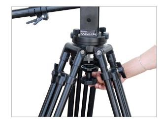
**NOTE:** It is important to make sure that the Central Fork is seated in the bowl properly. That means perpendicular to the tripod bowl. Off axis installation may hamper movement of the jib. Also you may need the assistance of a grip stand to hold the camera end of the arm during installation preventing it from falling as it will be front heavy at this point. You may also need the grip stand or assistance at the rear of the jib when mounting the camera.
