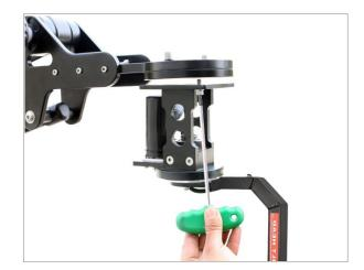
Now, mount your camera with camera mounting screw on Pan Tilt Head.
