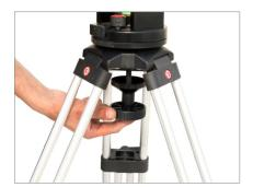
**NOTE:** Ensure that the Central Fork is seated in the bowl properly, i.e., perpendicular to the tripod bowl. Off-axis installation may hamper the jib movement. Also, you may need a grip stand to hold the camera end of the arm during structure, preventing it from falling as it will be front-heavy. You may also require the grip stand or assistance at the rear of the jib when mounting the camera.
