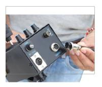
CAUTION: The power specification we have provided is as per 12volt. For this, we provide a 12volt/3ampere regulated power adapter. In case you use a voltage higher than 12V, it will affect the performance and life of the motor, and there is a high risk of the motor getting damaged.
